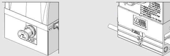
Air outlet adjusted to the next bases. Front outlet closed, however usable by removing the cap from the fitting.
