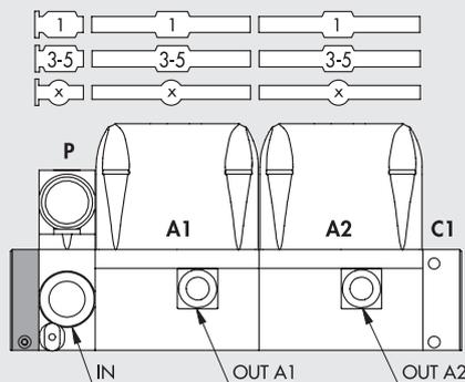
Island consisting of a single pneumatic supply (P) and front outlet from individual regulators.
