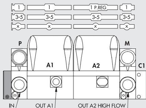
Hybrid island. It consists of regulators with a local output (A1) and in-series high-flow rate regulators via intermediate element M downstream of regulator A2. Power supply P is in common.
