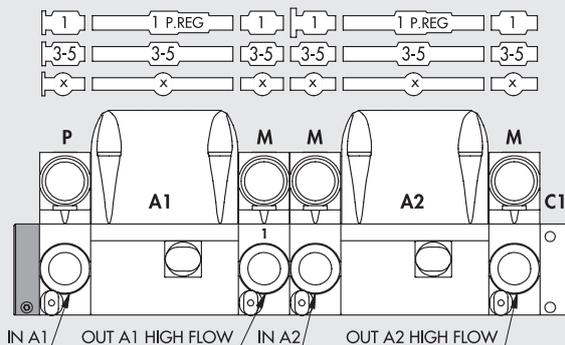
Island consisting of independent regulator power supply, via P supplies and intermediate elements M (with port 1 closed) placed upstream of the regulator. High-flow outputs are obtained via intermediate elements M placed downstream of the individual regulators.
