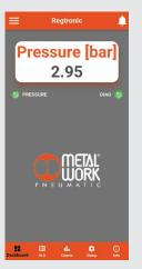
The Metal Work RegUp App can be used for connection via Bluetooth to Metal Work proportional pressure regulators in the REGTRONIC series with a wireless interface, from Android smartphone and iOS.
